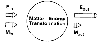
Fig. 1.1: Schematic depiction of matter and energy flow in a matter-energy transformation device. The length of the arrows is to suggest a decrease in mass flow, M_{out} < M_{in} , with a corresponding increase in energy flow, E_{out} > E_{in} .
