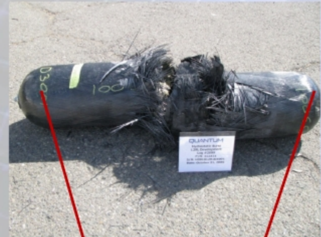
The localized reinforcement protected the dome regions very well
