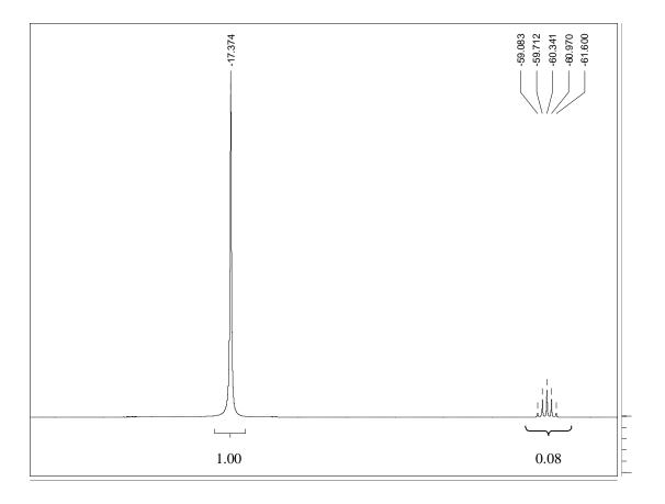
B<sup>11</sup> NMR of 1 ml 30 wt% NaBH<sub>4</sub> in 1M aqueous NaOH with catalyst in after 3 weeks Mass of catalyst = 0.02g (5% Ru on alumina), Boric Acid: 0 ppm.
