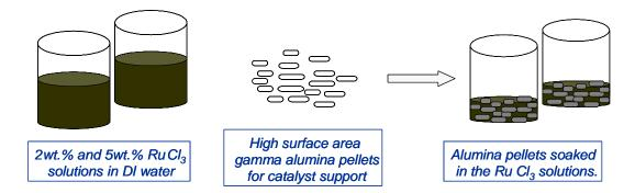
Solution soaked  $RuCl_3$  on alumina pellets, decanted, air dried. Samples were heated under 5% hydrogen, balance helium. heated at 100°C/hr to 150°C or 700°C, no dwell and 6 hour dwell
