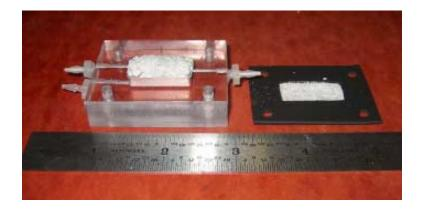
Alumina-borate solid lump that forms in hydrogen generation reactor from alumina dissolution 30wt% sodium borohydride in aqueous 1M NaOH solution.
