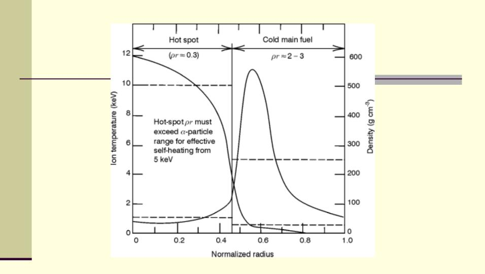
Fig. 3 Radial profiles of the ion temperature and density in a DT pellet computed at highest compression for an isobaric spark ignition [13] case according to Storm et al [41]. The radius of the fusion detonation wave is at 0.47 of the actual plasma radius and the dashed lines are the average temperature of inner and outer parts and the dashed-dotted lines are the averages of the densities respectively.
